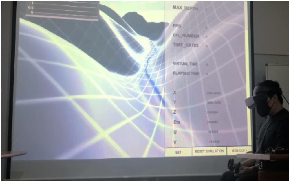
Figure 4.15: Snapshot of the VR experience within the numerical domain during the rainfall-runoff simulation on the GCEW
